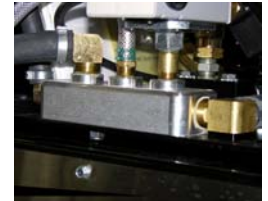
Manifold Assembly: Fewer connections and easier accessibility
