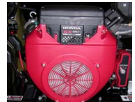
20 HP Honda Engine: OHV V-Twin horizontal shaft
